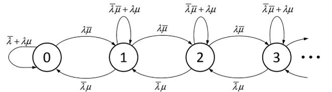
Figure 2: Markov chain for the sender's queue size – single receiver case. Here  $\bar{\lambda} := (1 - \lambda)$  and  $\bar{\mu} := (1 - \mu)$ .
