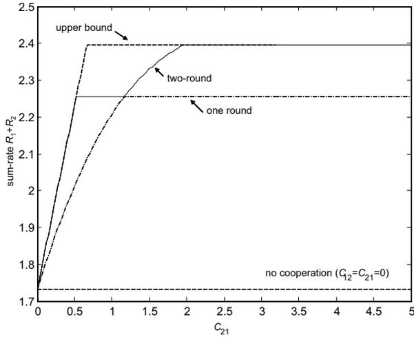
Fig. 3. Sum of the private rates  $R_1 + R_2$  (with  $R_0 = 0$ ) versus the conferencing link capacity  $C_{21}$  for the outer bound, the one-round and two-round strategies and with no cooperation ( $P_1 = P_2 = 10dB$ ,  $\gamma_{12}^2 = 0dB$ ,  $\gamma_{22}^2 = 0dB$ ,  $\gamma_{21}^2 = -3dB$ ,  $\gamma_{11}^2 = -3dB$ ,  $C_{12} = 0.2$ ).
