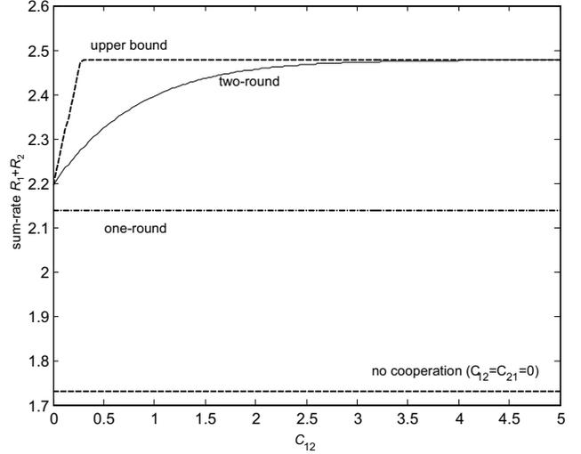
Fig. 4. Sum of the private rates  $R_1 + R_2$  (with  $R_0 = 0$ ) versus the conferencing link capacity  $C_{12}$  for the outer bound, the one-round and two-round strategies and with no cooperation ( $P_1 = P_2 = 10dB$ ,  $\gamma_{12}^2 = 0dB$ ,  $\gamma_{22}^2 = 0dB$ ,  $\gamma_{21}^2 = -3dB$ ,  $\gamma_{11}^2 = -3dB$ ,  $C_{21} = 0.8$ ).
