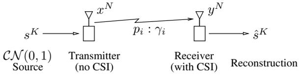
Fig. 1. Source-channel coding without CSI at the transmitter.
