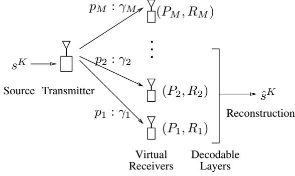
Fig. 2. Layered broadcast coding with successive refinement.
