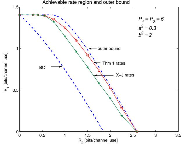
Fig. 5. Rates of Thm. 1 and [7, Thm.5] and outer bound of Cor. 1. Also shown is the capacity region of BC from the cooperating encoder,  $P_2 = 0$ .
