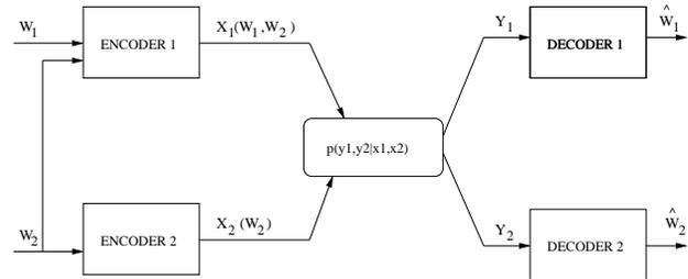
Fig. 1. Interference channel with cooperating encoder.
