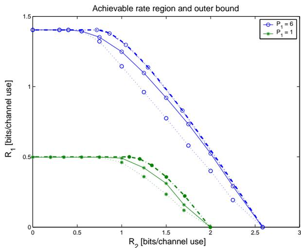
Fig. 7. Impact of reduced power of the cognitive transmitter to achievable rates. Rates achieved with Thm. 1 are shown in solid lines and rates of [7] are shown with dotted line. Dash-dotted line shows the outer bound.
