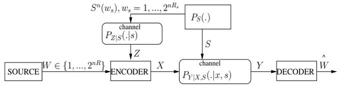
Fig. 4. Channel with an interfering codeword observed through a noisy channel at the cognitive encoder.
