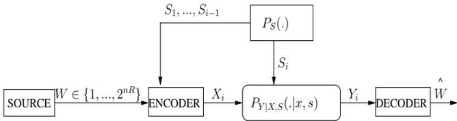
Fig. 3. Channel with random states known with delay at the transmitter.
