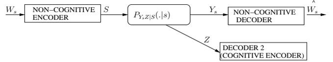
Fig. 6. Channel from the interferer to its receiver and to the cognitive encoder (labeled decoder 2).
