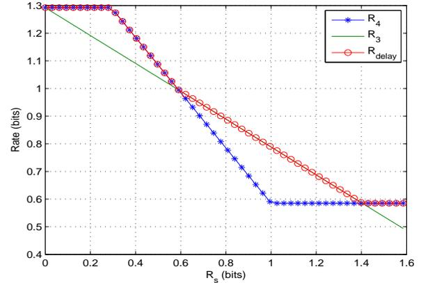
Fig. 8. Performance when the cognitive encoder learns the interferer's sequence causally with noise in the Gaussian channel with a Gaussian codebook at the interferer.
