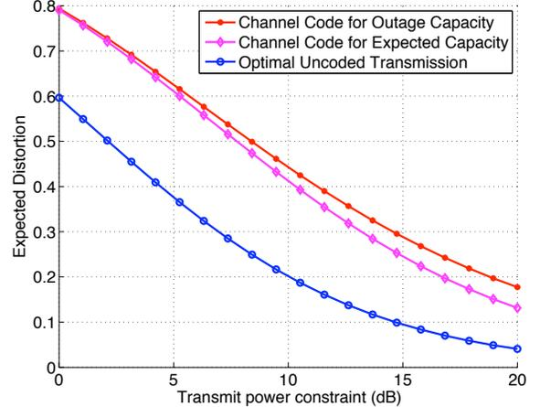
Fig. 3. Expected distortion for various source-channel coding schemes
