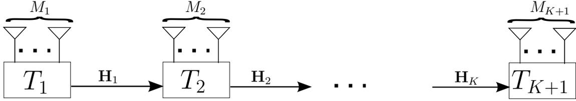
Fig. 1. The  $(M_1, M_2, \dots, M_{K+1})$  MIMO multi-hop relay network. Each terminal can receive only the signal transmitted by the terminal preceding itself in the network.
