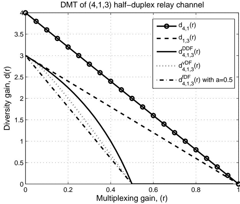
Fig. 3. The DMT curve of a (4, 1, 3) multi-hop relay channel. The two topmost curves correspond to the cut-set bounds, where the dashed curve is also the DMT for a full-duplex relay. The DDF, vDF and fDF protocol with  $a = 0.5$  are also illustrated, where the DDF curve is the optimal DMT with half-duplex relaying.
