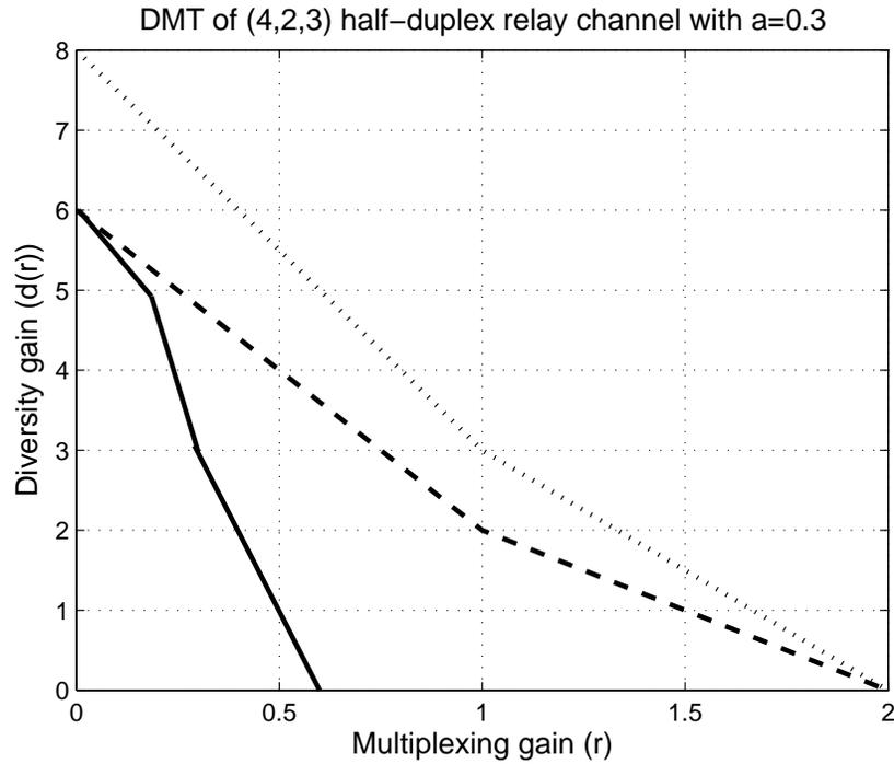
Fig. 2. The dotted and the dashed curves correspond to  $d_{4,2}(r)$  and  $d_{2,3}(r)$ , respectively. Note that the dashed curve also corresponds to the DMT in the case of a full-duplex relay terminal. The solid curve is the DMT curve of a  $(4, 2, 3)$  half-duplex multi-hop relay with fDF protocol and  $a = 0.3$ .
