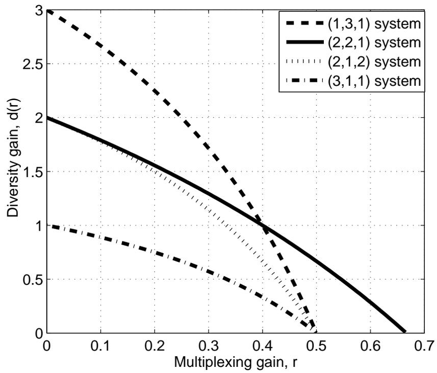
Fig. 5. The DMT of all 2-hop multi-hop MIMO systems that are possible with a total of 5 antennas.
