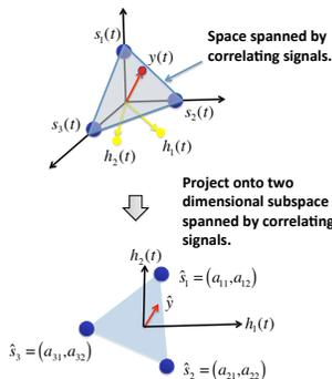
**Fig. 3:** The projection performed by RD-MUD. The figure illustrates the case  $N = 3$ ,  $M = 2$ , and the received signal is due to two active users.
