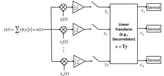
Fig. 1: Conventional MUD using a bank of MFs.
