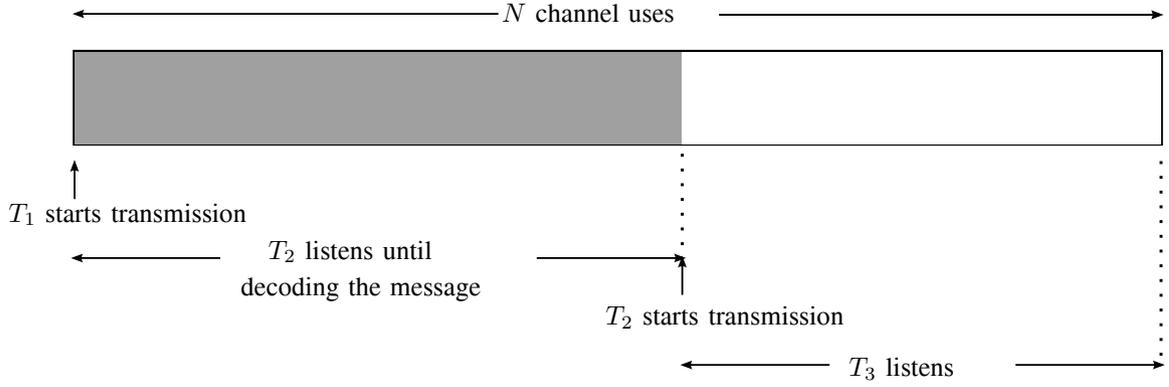
Fig. 4. Illustration of the DDF protocol for a single relay multihop network.
