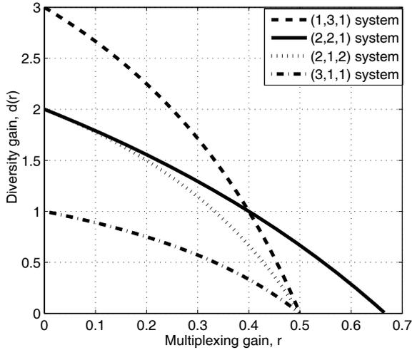
Fig. 6. The DMT of all 2-hop MIMO systems that are possible with a total of 5 antennas.
