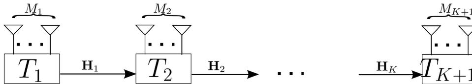
Fig. 1. The  $(M_1, M_2, \dots, M_{K+1})$  MIMO multi-hop relay network. Each terminal can receive only the signal transmitted by the terminal preceding itself in the network.
