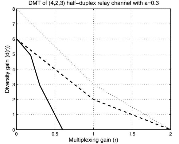
Fig. 2. The dotted and the dashed curves correspond to  $d_{4,2}(r)$  and  $d_{2,3}(r)$ , respectively. Note that the dashed curve also corresponds to the DMT in the case of a full-duplex relay terminal. The solid curve is the DMT curve of a  $(4, 2, 3)$  half-duplex multi-hop relay with fDF protocol and  $a = 0.3$ .
