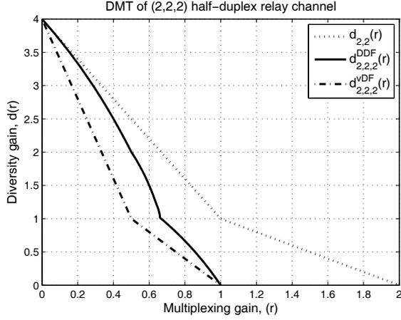
Fig. 5. The DMT of a  $(2, 2, 2)$  system. From top to bottom, the three curves correspond to the full-duplex relay DMT, the half-duplex relay DMT which is achievable by DDF protocol, and the DMT of the static protocol with  $a = 0.5$ .
