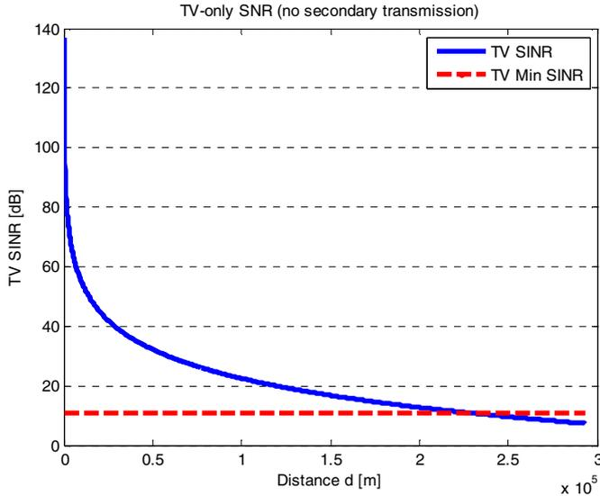
Figure 5. SINR of the TV signal over distance from the TV transmitter.
