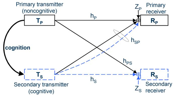
Figure 1. Cognitive radio channel.
