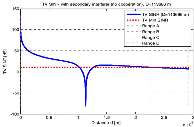
Figure 16. TV SINR over distance with a BS displacement of ~113 km and without cognitive relaying at the BS.
