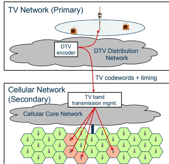
Figure 4. Coupled primary and secondary transmission networks (cellular radio cells with cognitive secondary transmission are marked in red).
