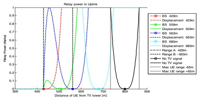
Figure 23. BS relay power vs. UE distance for different BS locations.
