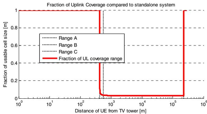
Figure 25. Performance loss of secondary uplink transmission.
