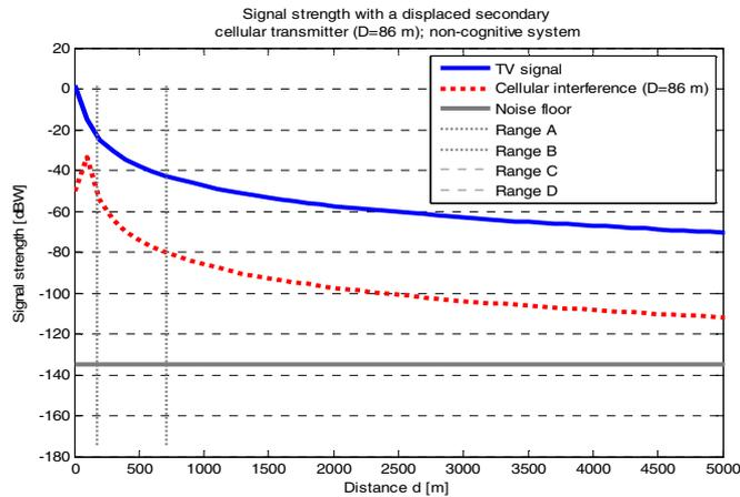
Figure 12. TV and cellular signal power over distance from TV transmitter with a BS displacement of 86 m.
