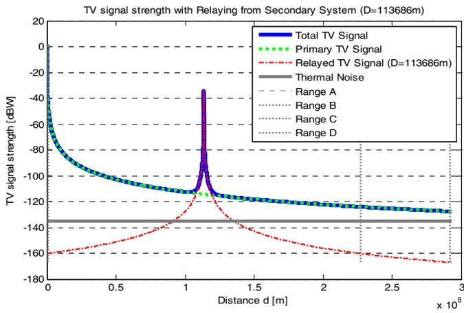
Figure 14. TV signal power over distance from TV transmitter with a cognitive relaying from a BS by ~113 km.
