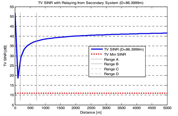
Figure 13. TV SINR over distance with a BS displacement of 86 m.
