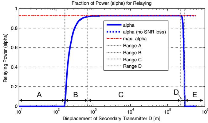
Figure 11. Required relay power vs. displacement of BS from TV transmitter.
