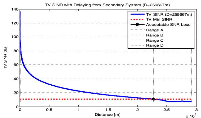
Figure 19. TV SINR with cognitive relaying from the BS in region D and an acceptable SNR loss at the TV service area edge.
