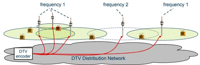
Figure 3. Architecture of a digital TV system.
