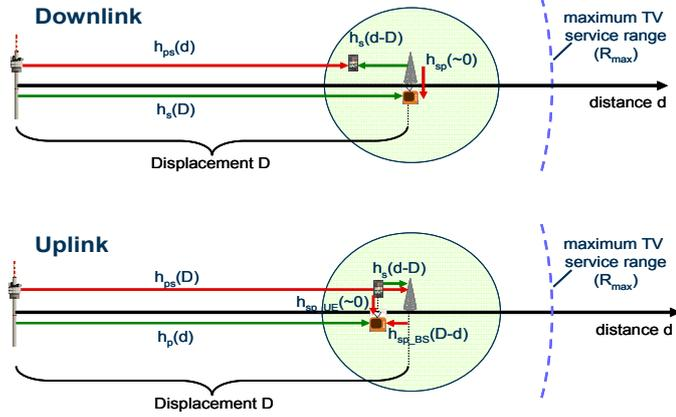
Figure 9. Simulation model within TV service area and  $h(r)$  depending on distance  $r$  between transmitter and receiver.
