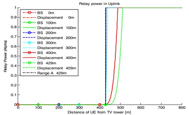
Figure 21. BS relay power vs. UE distance for different BS locations.
