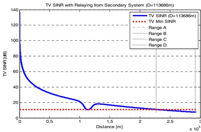
Figure 15. TV SINR over distance with a BS displacement of ~113 km and cognitive relaying from the BS.
