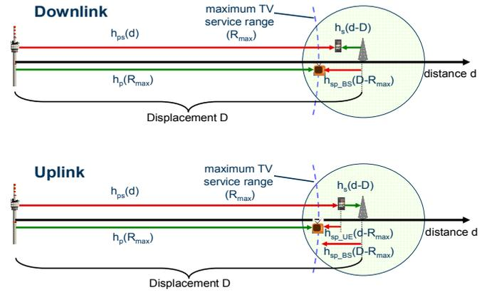
Figure 10. Simulation model outside TV service area.
