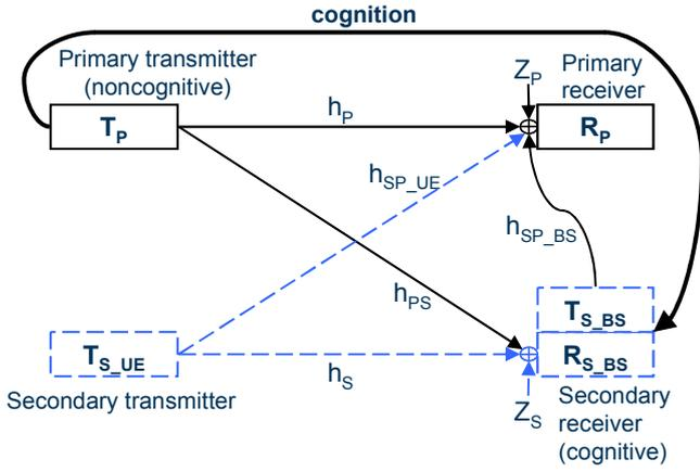
Figure 6. Channel model for the cognitive cellular uplink.
