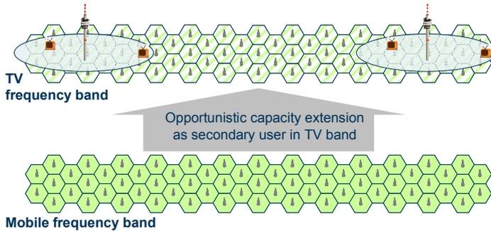
Figure 2. Usage scenario for secondary cognitive transmission.
