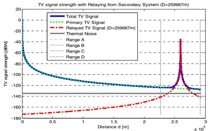
Figure 18. TV signal power over distance from TV transmitter with a cognitive relaying from a BS in region D.
