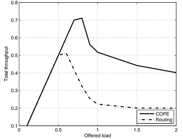
Fig. 6. Throughput for COPE and non-COPE systems in a cross network with cross traffic and traffic generated at the center node.
