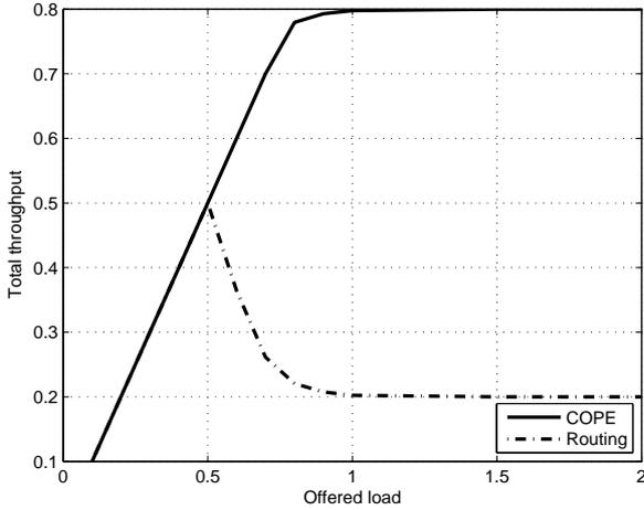
Fig. 5. Throughput for COPE and non-COPE systems in a cross network with cross traffic only.
