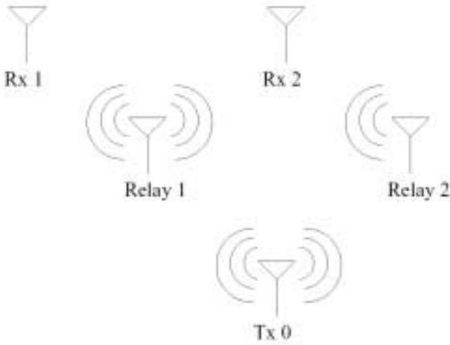
Fig. 2. A wireless relay communication scenario. A single transmitter, Tx 0, sends a message intended for two receivers Rx 1 and Rx 2 via multi-hop transmission. The two intermediate relay nodes each decode the message, re-encode, and transmit to the ultimate destination. Rx 1 sees only the signal from Relay 1, while Rx 2 receives potentially interfering signals from both relays.
