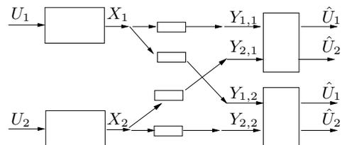
Fig. 1. Transmitting Correlated Sources over a Broadcast Network. Two correlated sources  $U_1$  and  $U_2$  are observed by independent transmitters and both sources must be communicated to each receiver.
