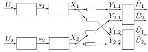
Fig. 3. Channel Figure with Separate Source-Channel Encoding and Joint Source-Channel Decoding
